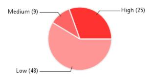
From this pie chart, you can obtain a graphical visualization of the defect distribution by impact. You can find at a glance whether the defects that Polyspace Bug Finder found in your code are low-impact defects. For more information on impact, see "Classification of Defects by Impact" on page 5-7.
